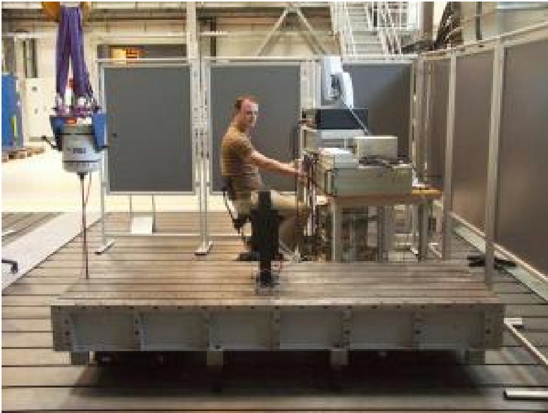
The round vibration exciter (left), suspended from a crane, induces vibrations in the rectangular iron platform that are similar to those of a wind energy converter. The active damper -- located at the center of the platform -- reduces these vibrations. (Credit: Copyright Fraunhofer IWU)
